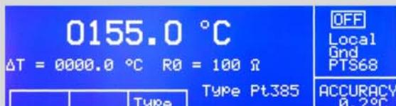
For temperature sensor simulation one of temperature scales PTS68 or ITS90 can be selected. Two types of Pt temperature sensors are predefined, PT 1.385 and PT 1.392.
