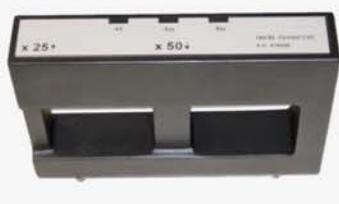
Option 140-50 Current coil with multiplying coefficient x25 and x50 is a usefull tool for calibration of clamp ammeters up to 1000 A at 50/60 Hz signal frequency.
