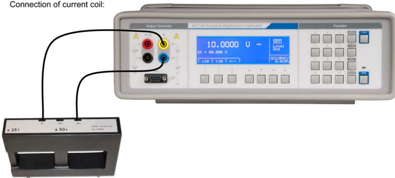
Fig. 25 Current coil connection
